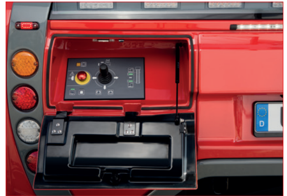
Supporting control panel with cover
